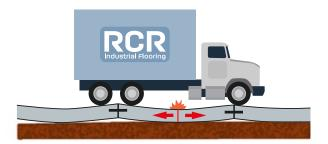
The position of sawn joints dividing the concrete slab in small panels is defined such as only one set of wheels can load one individual panel at any time. This results in a drastic reduction of stresses and tensions in the concrete.
